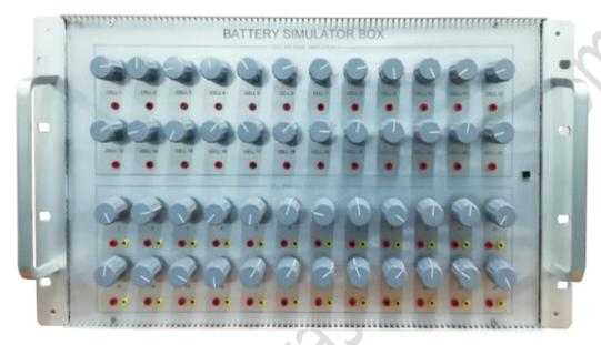
The Battery Cell Simulator/BMS Tester is designed to replicate the electrical and environmental conditions that battery cells experience during normal operation. It allows comprehensive testing of the BMS's functions, such as cell voltage monitoring, current sensing, temperature monitoring, state of charge estimation, and cell balancing.
