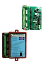
An elevator floor audio annunciator, also known as a voice announcement system, is a feature commonly found in elevators that provides auditory cues to indicate the current floor. It is designed to assist passengers, especially those with visual impairments, in identifying the floor they are on and navigating within a building. It also has pleasant Background music during a lift in operation.
