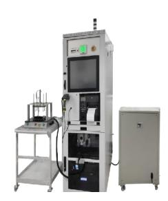
The PCBA EOL tester is designed to validate the operation of the entire PCB assembly, including the components, interconnections, and integrated circuits. It performs a series of functional tests and measurements to ensure that the PCBAs meet the required specifications and standards. The EOL tester may include various hardware and software components to facilitate comprehensive testing.
